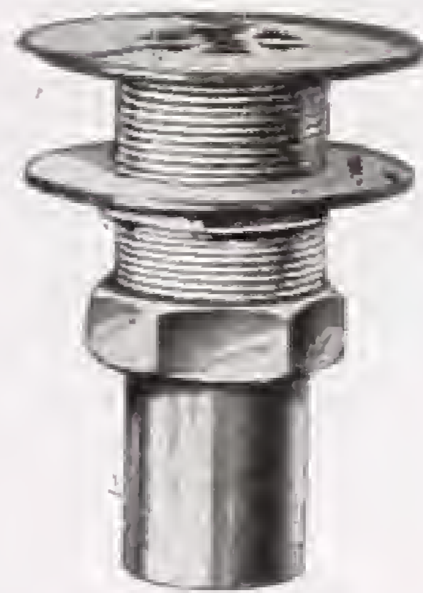
No. B 955 SINK WASTE With flush grating. With backnut and straight union. Sizes : 1 1/2 in., 2 in.
